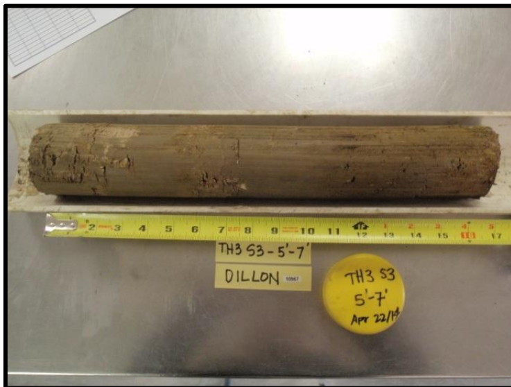
Figure 4: Borehole TH3 Hydraulic Conductivity Sample (approximately 2.0 m below ground level)
